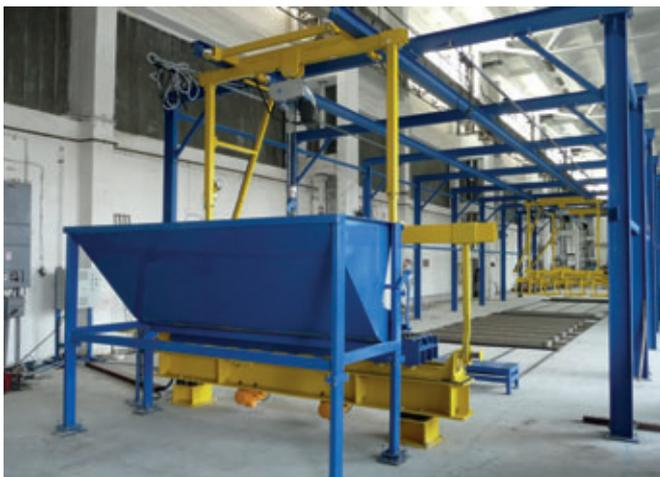
*L-3 production system with Knauer vibration station; the system was sold in the region around Budapest by the Hungarian company Atillas, for nearly 20 years the professional partner for the concrete industry in Hungary, Ukraine and Romania ([www.atillas.hu](http://www.atillas.hu)).*
