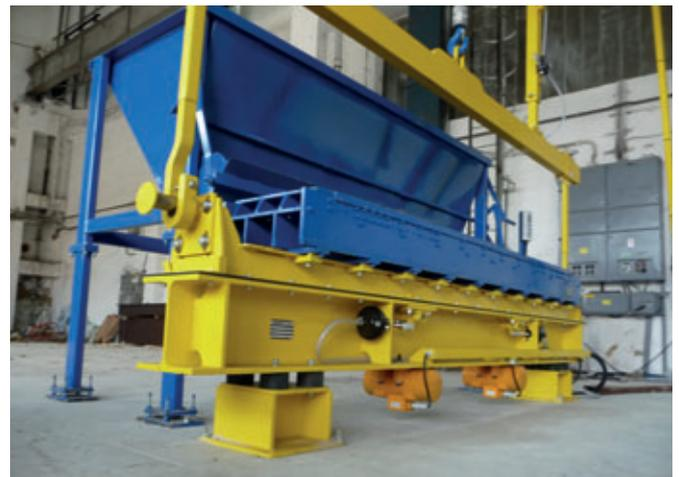
*Vibration table with two motors and pneumatic clamping*
